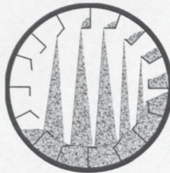
Figure A1.18 Typical flight arrangement, rotary cascade dryer
