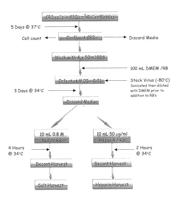
Figure 5.12 Flow diagram of virus growth and harvesting methods salt or heparin.
