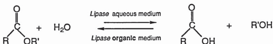
Scheme 5. The reversibility of lipase-catalysed reactions.
