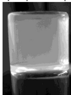
Figure 2. Vial-inversion demonstrating a lack of flow and hence the formation of a gel. Taken from Adams et al. 71 Reproduced by permission of The Royal Society of Chemistry
