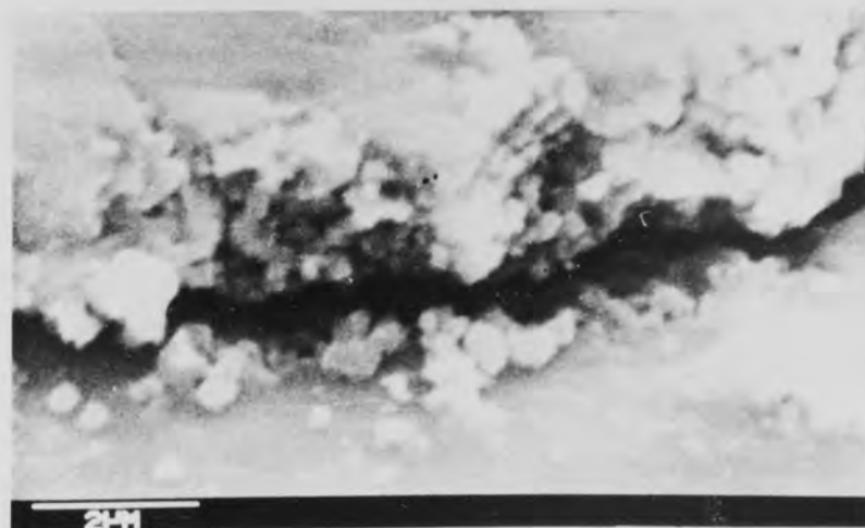
FIG. 4.9 SCANNING ELECTRON MICROGRAPHS OF SURFACES AFTER THE ESTABLISHMENT OF MILD WEAR CONDITIONS IN THIS CASE FOR AN EXPERIMENT CONDUCTED AT 120 mm/s, 22N LOAD AND TEMPERATURE OF 300 C.
