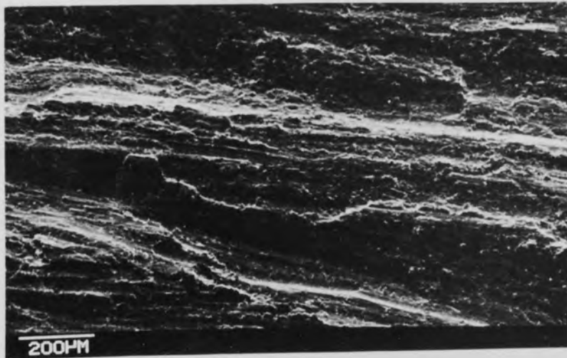
FIG. 4.8 SCANNING ELECTRON MICROGRAPH OF TYPICAL SEVERE WEAR SURFACE.
