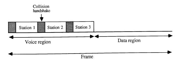
Figure 4.13b Ethernet-type compatible Logical TDMA
