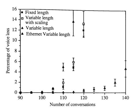
Figure 4.18 Percentage of voice loss at various voice loads using Logical TDMA with a voice region of 7.44ms.
