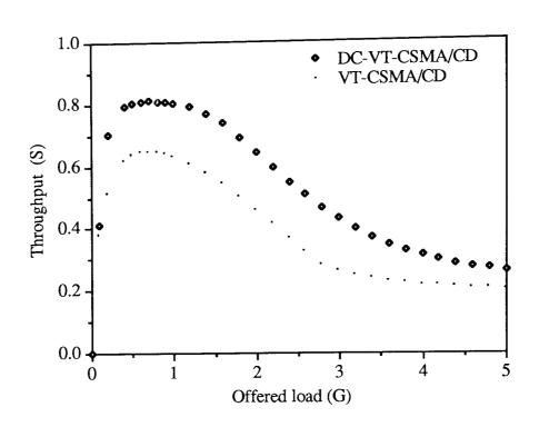
Total channel capacity =10Mbps, signalling channel =100Kbps, end-to-end propagation delay = 10 $\mu$ s, 1000 bit packets and  $\eta$ =7.
