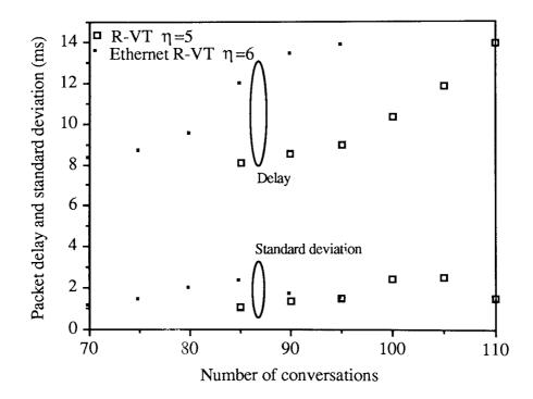
Figure 3.14 Packet delay and delay standard deviation using bit loss R-VT-CSMA/CD with binary exponential backoff with established user preemption
