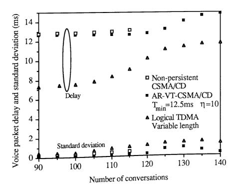
Figure 4.22 Voice packet delay and standard deviation of delay at various voice loads using CSMA/CD, AR-VT-CSMA/CD and Logical TDMA.
