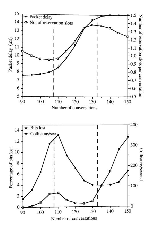
Figure 4.7 The performance of AR-VT-CSMA/CD when  $\eta=8$  and Tmin=7.5ms and Tmax=15ms.
