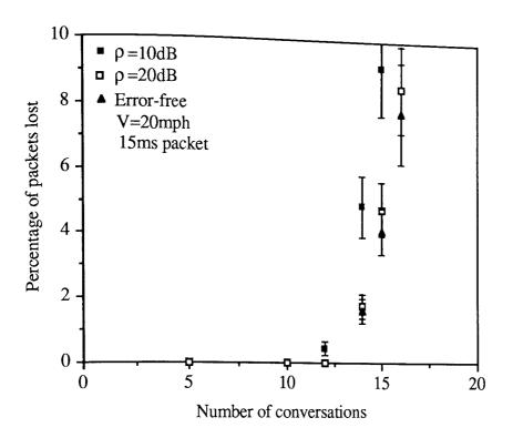
Figure 5.19 Percentage of voice packets lost for various voice loads using Logical TDMA over mobile radio with fixed length packets.
