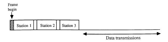
Figure 4.13a Standard Logical TDMA
