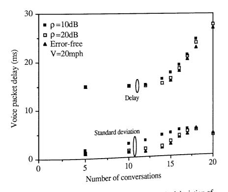
Figure 5.22 Voice packet delay and standard deviation of delay for various voice loads using Logical TDMA with variable length packets over mobile radio channels.
