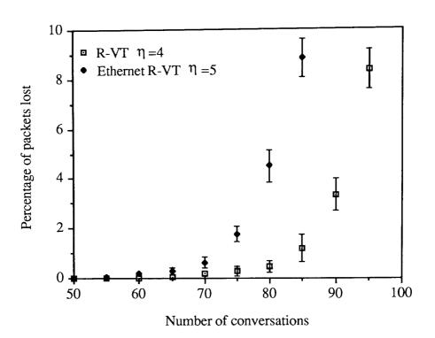
Figure 3.7 Percentage of packets lost using R-VT-CSMA/CD with a uniform collision backoff.
