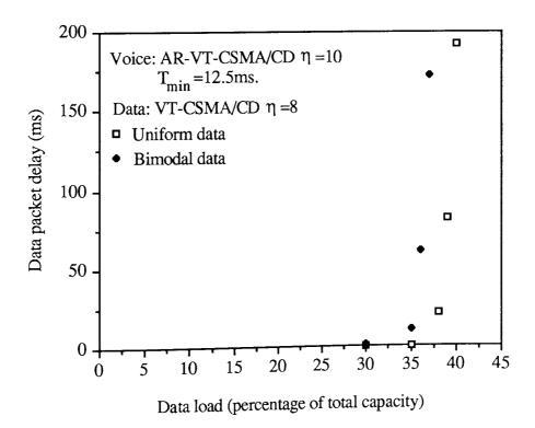
Figure 4.12 Data packet delay at various data loads and for a constant voice load of 40 conversations.
