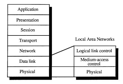
Figure 1.1 LAN standards apply to the data link and physical layers of the OSI reference model.
