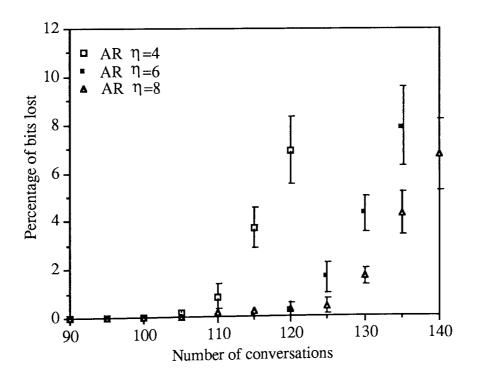
Figure 4.4 Percentage of voice bits lost using AR-VT-CSMA/CD with Tmin=10ms and Tmax=15ms.
