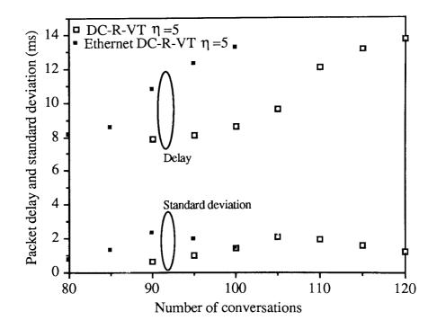
Figure 3.26 Packet delay and delay standard deviation using DC-R-VT-CSMA/CD with binary exponential backoff and established station preemption.
