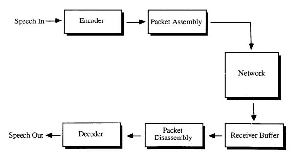
Figure 2.1 The voice packet process.
