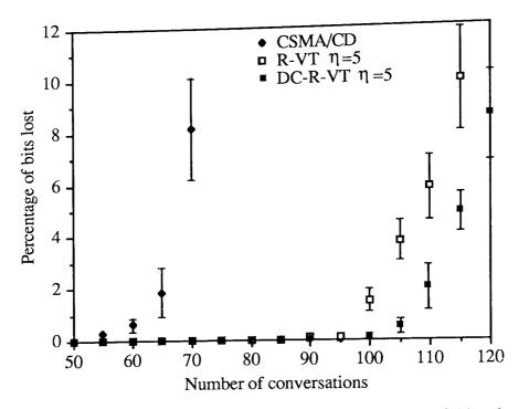
Figure 3.29 A comparison of the percentage of bits lost for the CSMA/CD, R-VT-CSMA/CD and DC-R-VT-CSMA/CD protocols.
