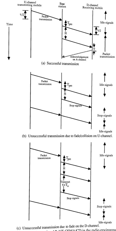
Figure 5.8 Packet transmissions using AR-VT-CSMA/CD in the radio environment.
