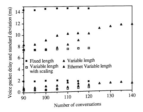
Figure 4.19 Voice packet delay and standard deviation of delay at various voice loads using Logical TDMA with a 7.44ms voice region.
