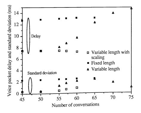
Figure 4.17 Voice packet delay and standard deviation of delay at various voice loads using Logical TDMA with a 3.76ms voice region.
