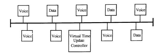
Figure 3.3. Schematic of Ethernet-type compatible R-VT-CSMA/CD
