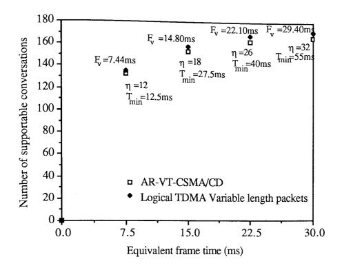
Figure 4.23 Number of supportable conversations, assuming 2% bit loss is acceptable, for AR-VT-CSMA/CD and Logical TDMA at various equivalent frame times.
