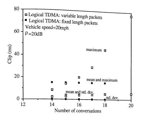
Figure 5.23 Mean, maximum and standard deviation clip statistics with Logical TDMA over mobile radio channels using fixed and variable length packets.
