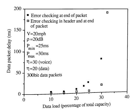
Figure 5.13 Data packet delay at various data loads with a constant voice load of 10 conversations.
