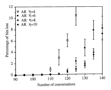
Figure 4.6 Percentage of voice bits lost using AR-VT-CSMA/CD with Tmin=14.9ms and Tmax=15ms.
