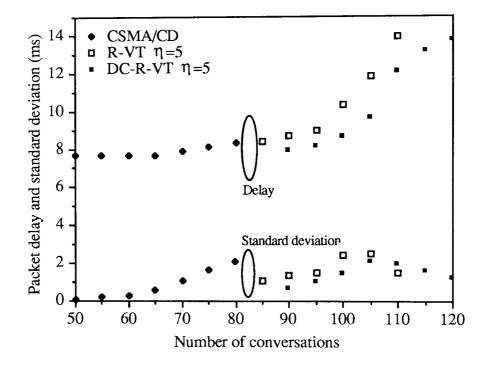
Figure 3.30 A comparison of the packet delay and standard deviation for the CSMA/CD, R-VT-CSMA/CD and DC-R-VT-CSMA/CD protocols.
