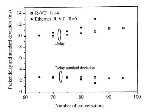
Figure 3.9 Packet delay and delay standard deviation using R-VT-CSMA/CD with a uniform collision backoff
