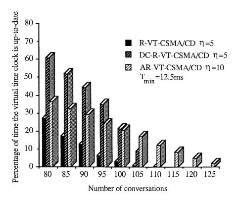
Figure 4.11 A comparison between R-VT-CSMA/CD, DC-R-VT-CSMA/CD and AR-VT-CSMA/CD of the amount of time the virtual time clock is up-to-date with the real time clock.
