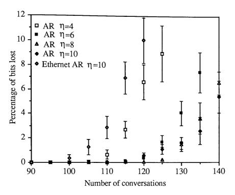
Figure 4.5 Percentage of voice bits lost using AR-VT-CSMA/CD with Tmin=12.5ms and Tmax=15ms.
