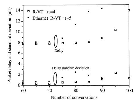
Figure 3.12 Packet delay and delay standard deviation using R-VT-CSMA/CD with binary exponential backoff and established user preemption.
