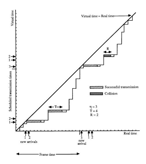
Figure 3.2. Collisions can occur between established voice stations in R-VT-CSMA/CD.
