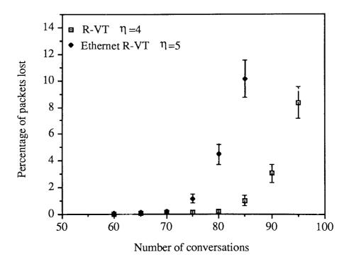
Figure 3.8 Percentage of packets lost using R-VT-CSMA/CD with a binary exponential collision backoff.
