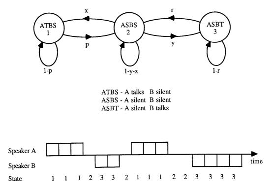
Figure 6.3 3-state Markov chain model, with possible sequence of states.
