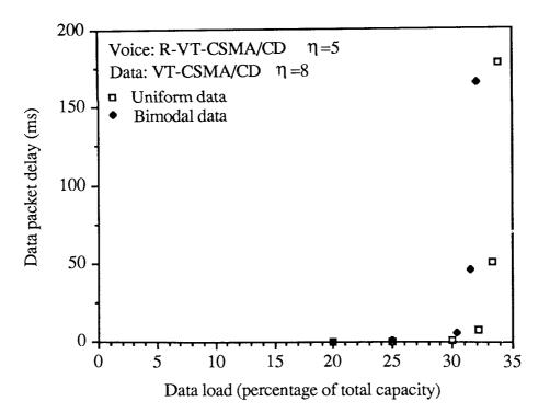
Figure 3.15 Data packet delay at various data loads with a constant voice load of 40 conversations.
