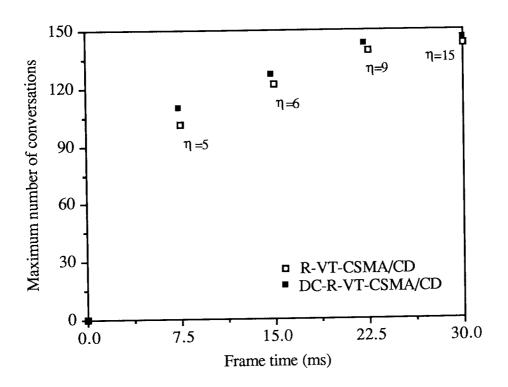
Figure 3.31 Number of conversations for 2% bit loss using R-VT-CSMA/CD and DC-R-VT-CSMA/CD at various frame times.
