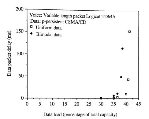
Figure 4.20 Data packet delay at various data loads with a constant voice load of 40 conversations.
