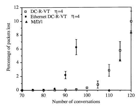
Figure 3.22 Percentage of voice packets lost using DC-R-VT-CSMA/CD with a binary exponential collision backoff and established station preemption.
