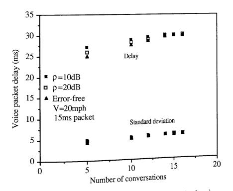
Figure 5.20 Voice packet delay at various voice loads using Logical TDMA over mobile radio with fixed length packets.
