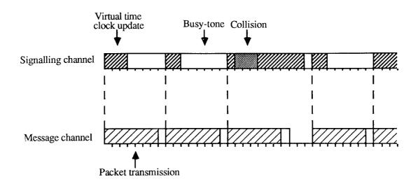
Figure 3.16 Timing diagram for R-VT-CSMA/CD with split-channel reservation
