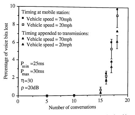
Figure 5.9 Percentage of voice lost at various loads, with mobile stations maintaining virtual time and with virtual time lag appended onto packet transmissions.
