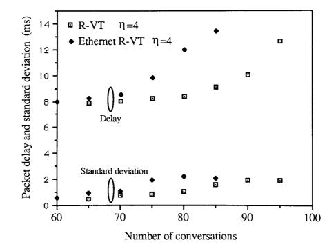
Figure 3.10 Packet delay and delay standard deviation using R-VT-CSMA/CD with a binary exponential collision backoff.
