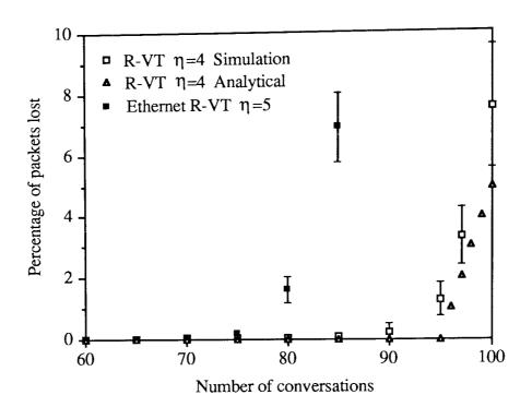
Figure 3.11 Percentage of packets lost using R-VT-CSMA/CD with a binary exponential collision backoff and established user preemption.
