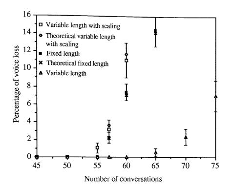
Figure 4.16 Percentage of voice loss at various voice loads using Logical TDMA with a voice region of 3.76ms.
