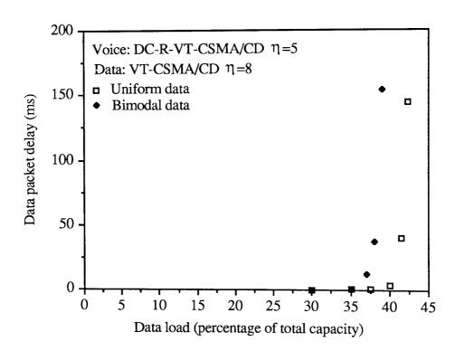
Figure 3.28 Data packet delay at various data loads and for a constant voice load of 40 conversations.
