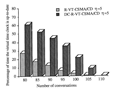
Figure 3.27 A comparison between R-VT-CSMA/CD and DC-R-VT-CSMA/CD of the amount of time the virtual time clock is up-to-date with the real time clock.
