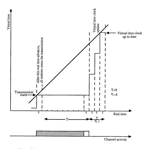
Figure 3.6. Virtual time clock update for synchronous VT-CSMA.
