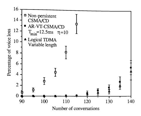
Figure 4.21 Percentage of voice loss at various voice loads using CSMA/CD, AR-VT-CSMA/CD and Logical TDMA.
