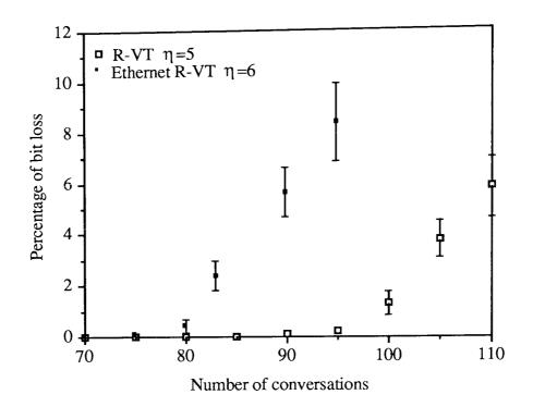
Figure 3.13 Percentage of bit loss using bit loss R-VT-CSMA/CD with binary exponential backoff and established user preemption.
