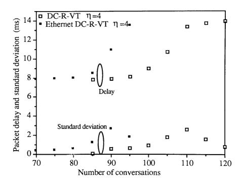
Figure 3.24 Voice packet delay and delay standard deviation using DC-R-VT-CSMA/CD with binary exponential collision backoff and established station preemption.
