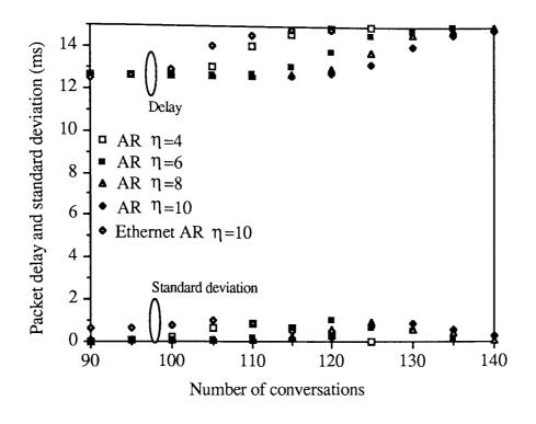
Figure 4.10 Packet delay and standard deviation using AR-VT-CSMA/CD with  $T_{min} = 12.5 \text{ms}$  and  $T_{max} = 15 \text{ms}$ .
