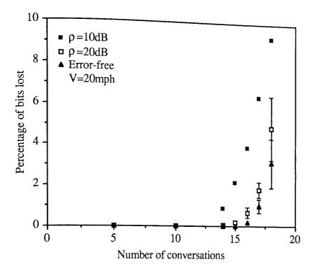
Figure 5.21 Percentage of bits lost using Logical TDMA with variable length packets over mobile radio channels.
