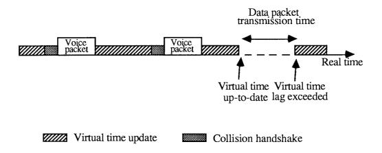
Figure 3.4. Timing diagram of Ethernet-type compatible R-VT-CSMA/CD. Virtual time update with the carrier is achieved through the controller.
