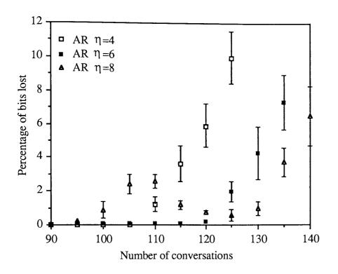
Figure 4.3 Percentage of bits lost using AR-VT-CSMA/CD with Tmin=7.5ms and Tmax=15ms.
