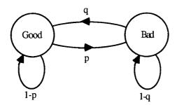
Figure 6.4 Gilbert model for mobile channel characteristics
