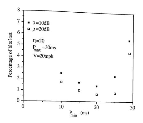
Figure 5.12 Variation of percentage of bits lost versus  $P_{min}$  with a constant voice load of 15 conversations.
