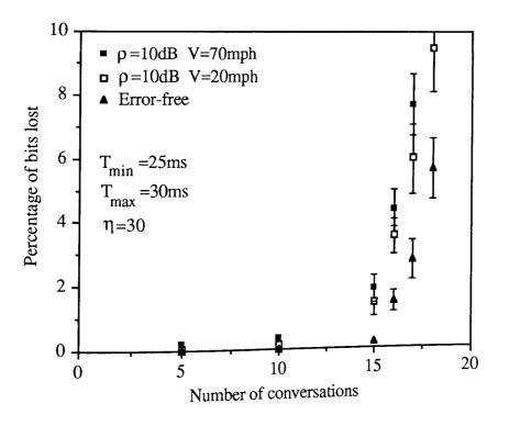
Figure 5.11 Percentage of bits lost at various voice loads using AR-VT-CSMA/CD for an error-free and 10dB SNR environment.
