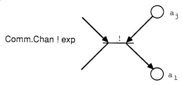
These two actions, input and output, always appear in pairs in the system. In systems which use a parallel processing language such as Occam where communications are synchronised, the same transition will be shared by both processes involved in the communication.
