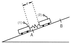
Figure 1.1 An example of a decentralised control system
