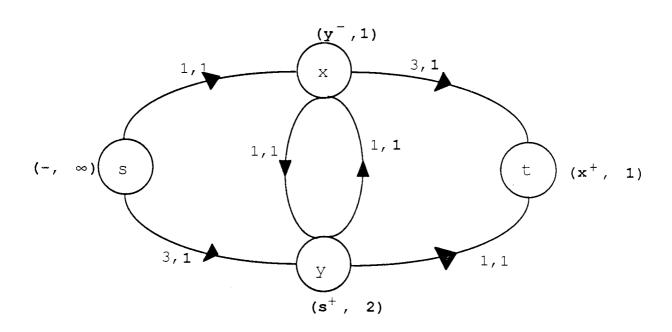
The final digraph shows that after re-application of routine B. The routine A is unable to find the flow augmenting path to sink, t.
