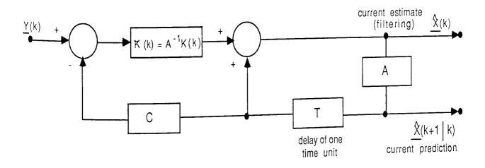
Figure 4.4 Simultaneous filtering and prediction of vector signals
