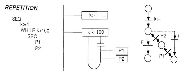
Fig. D1 Petri Net Models of Sequential Software Constructs.
