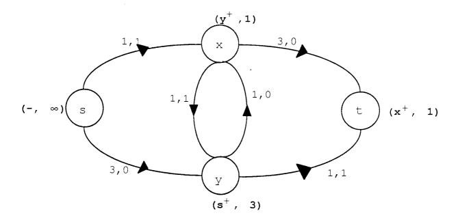
The next step in the process is to initiate **routine B**. The digraph shown below depicts the changes in the flow due to the routine and the re-application of **routine A** again. All the changes to the digraph are highlighted in bold characters.
