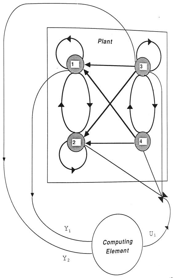
Figure 5.6 Graphical representation of state space equation of a control problem
