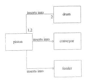
Fig. 6.5 Can sorting machine object diagram
