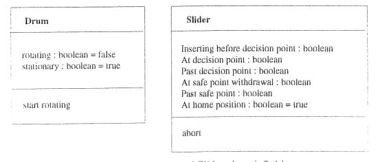
Fig. 3.20 Drum and Slider class definition
