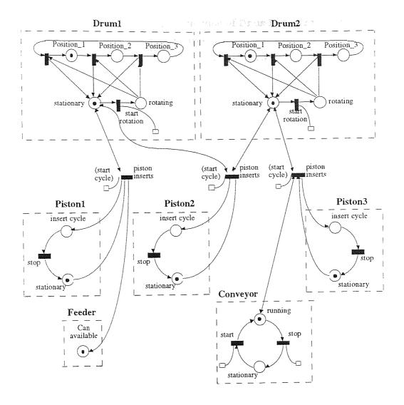
Fig. 6.8 The Petri net model representing the can sorting machine
