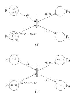
Fig. 2.23 Illustrating the firing rule for high level Petri nets
