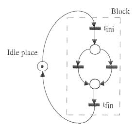
Fig. 3.3 Well formed block with idle place
