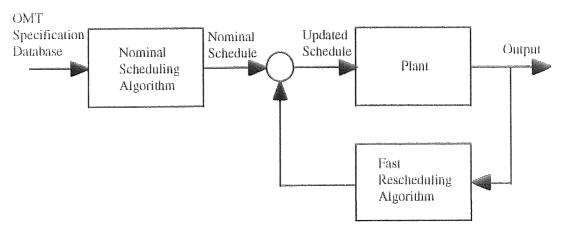
Fig. 4.21 Re-scheduling function of the re configurable controller
