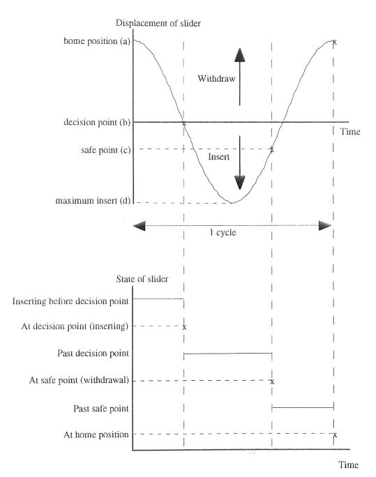
Fig. 3.19 Mapping a continuous motion to a set of discrete states
