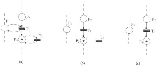
Fig. 2.15 Reduction R<sub>a</sub> (self-loop transition)
