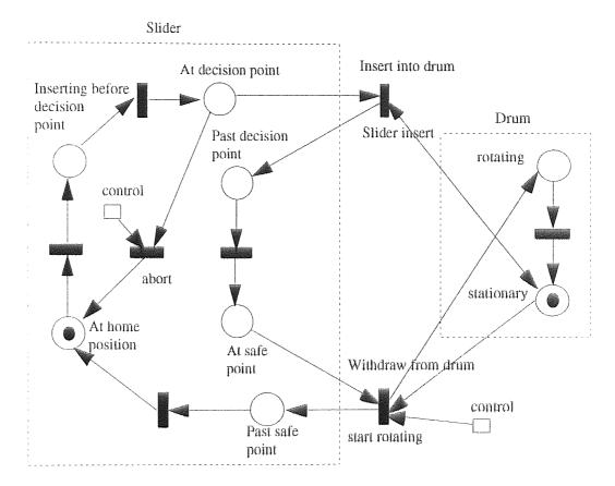
Fig. 3.23 The Drum-Slider Petri net
