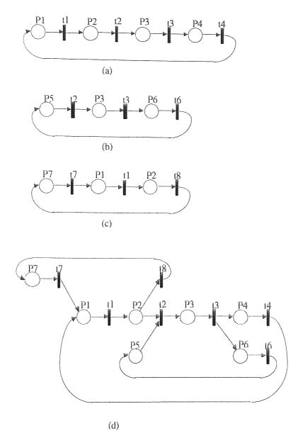
Fig. 3.2 (a)-(c) Three SECs, (d) Three SEC's combined along an STP and an SPP [Jeng and DiCesare 93]
