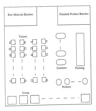
Fig. 6.11 Layout of a Semiconductor testing plant
