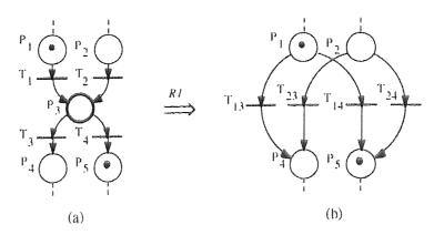
Fig. 2.20 Substitution of a place with more than one input and output [David and Alla 92]
