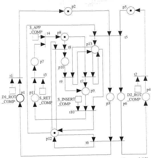
Fig. 6.10 CPN representation of can-sorting machine [Holding et al. 95]
