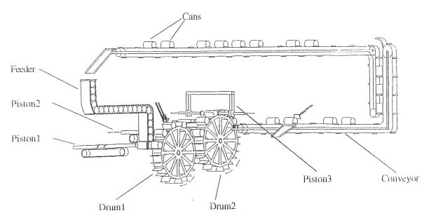
Fig. 6.1 Eurotherm controls prototype can sorting machine
