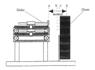
Fig. 3.17 The drum-slider mechanism
