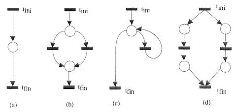
Fig. 3.4 Well formed blocks: (a) "Sequence" block; (b) "if-then-else" block; (c) "do-while" block; (d) "fork-join" block [Valette 79]
