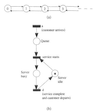
Fig. 2.8 Comparison of state diagram and Petri net
