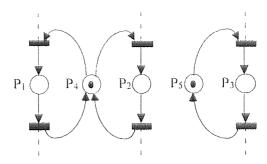
Fig. 4.24 Petri net representing section of production plant
