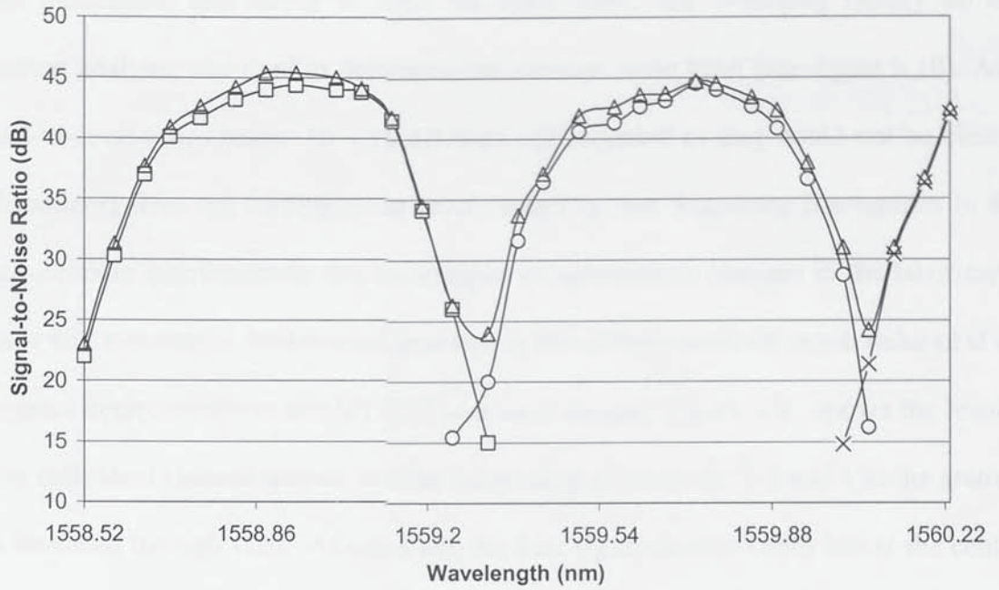
Figure 6.11 Signal to noise ratio vs. wavelength for the first FBG stretched through channel 3 to channel 1. Channel 3 (squares), channel 2 (circles), channel 1 (crosses) and 3+2+1 (triangles).
