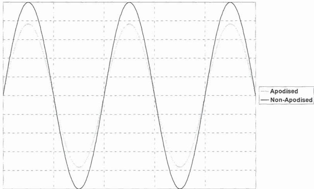
Figure 3-28: The effect of summing the three dephased fringe patterns shown in Figure 3-27, allowing a higher apodisation. The non-apodised graph is summated over three in-phase fringe patterns.
