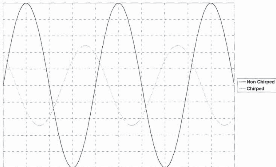
Figure 3-30: The effect of linearly dephasing three fringe patterns, in comparison with the summation of three in-phase patterns. The dephasing leads to a chirp effect.
