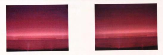
Figure 4.19 Photograph of the plasma-cathode sheath, 90 mT, 150 W, a)  $Ar + 50\% H_2$ , b)  $Ar + 75\% H_2$
