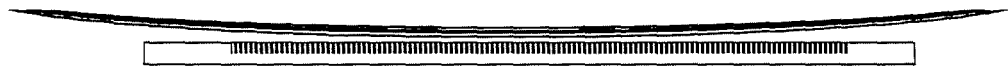
Figure 3.19: Placing the fibre very close to the phasemask can result in a bend in the fibre.
