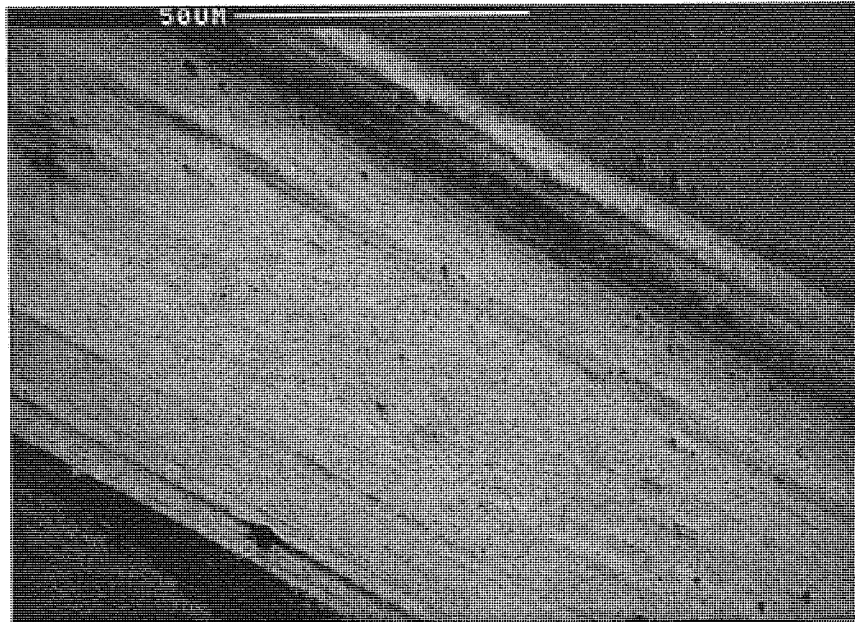
Figure 4.57 Wear Track on Tape ME#3 Resulting from Stop Motion Test
