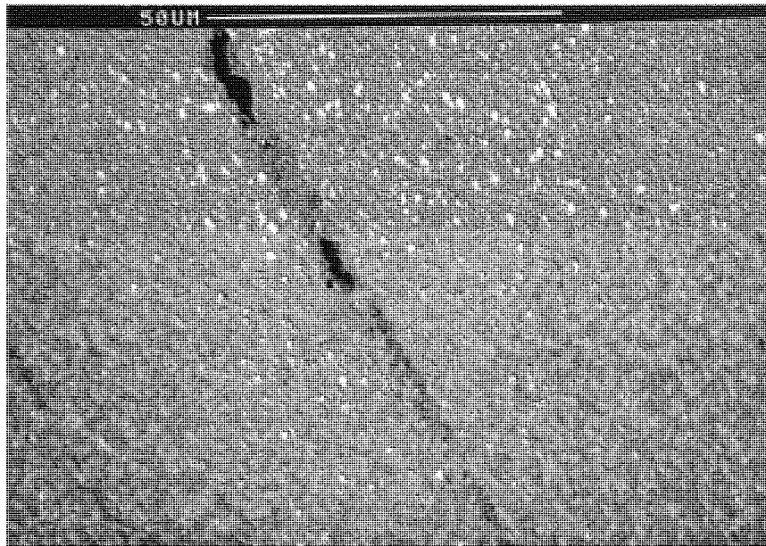
Figure 4.36 Wear scar Clearly Visible after 7 Hours of a Stop Motion Test at Ambient Conditions
