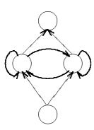
Figure 5: A schematic illustration of a recurrent network architecture used for speech recognition. The bias weights are not shown. The network discussed in the text used 22 input nodes, 176 hidden nodes, and 61 output nodes.
