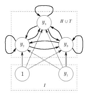
Figure 3: A recurrent network with 2 input nodes, including the bias node indicated by the "1". Any of the 3 non-input nodes could be a target or hidden node.
