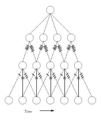
Figure 4: A simplified illustration of the structure of a Time Delay Neural Network (TDNN). Weights with corresponding markings have equal values. Therefore only 9 of the 27 weights shown are independent. The bias weights are not shown. Each node of this diagram would be replaced by a set of nodes in a realistic network.
