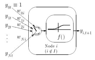
Figure 1: A non-input node of a neural network model containing N+1 nodes, including the bias node.
