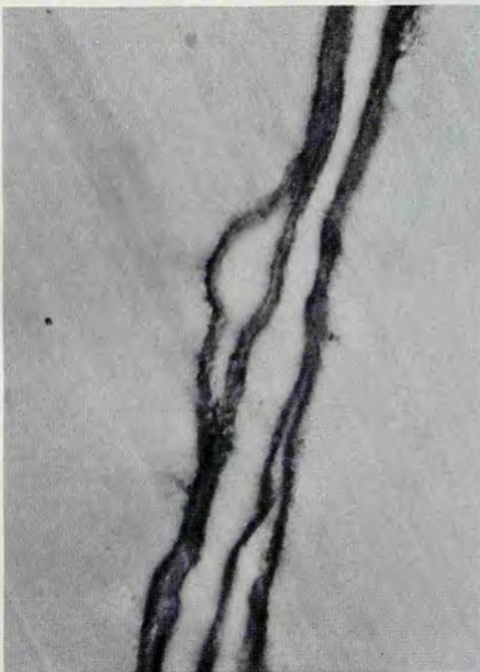
Plate 26. Boiled in bicarbonate solution Swollen, layered structure which has split at the middle lamella and within the wall. Individual fuzzy layers appear to be disintegrating further. x 10 000
