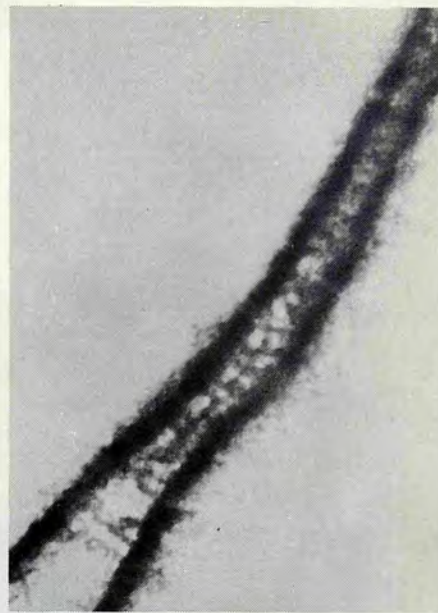
Plate 25. Boiled in water Middle lamella split and wall adopts a fuzzy appearance as material is dissolved. x 50 000
