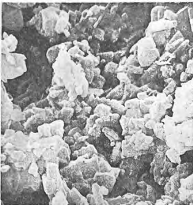
Plate 2 Upper Chalk from Yorkshire (721V; quarry face; a = 29.9 per cent; k = 1.2 md; d_{50} = 0.40 \mu\text{m} ). The field of view is about 15 \mu\text{m} .
