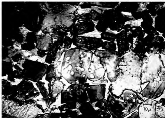
PLATE 4. Polished and etched surface of a Portland cement clinker, showing inclusions of \beta-C_2S in C_3S (centre and bottom right).
