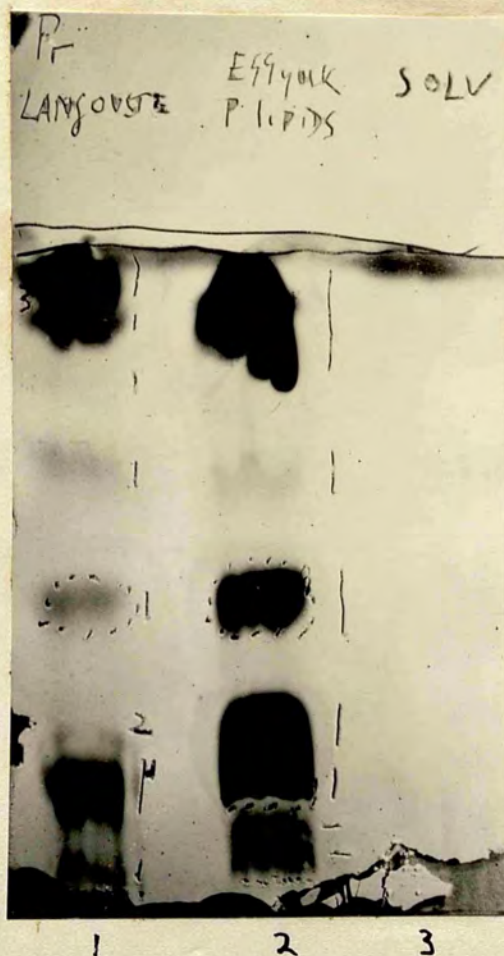
Figure 64. Thin-layer chromatography on silica gel G. Solvent: \text{CHCl}_3/\text{MeOH}/\text{H}_2\text{O} (80/30/3 v/v). Development distance: 10cm. Column 1. \text{CHCl}_3 -MeOH extract of the carotenoprotein of the ovary of P. vulgaris . Column 2. Hen's egg phospholipid Column 3. \text{CHCl}_3 -MeOH extract of Sephadex G25 (control).
