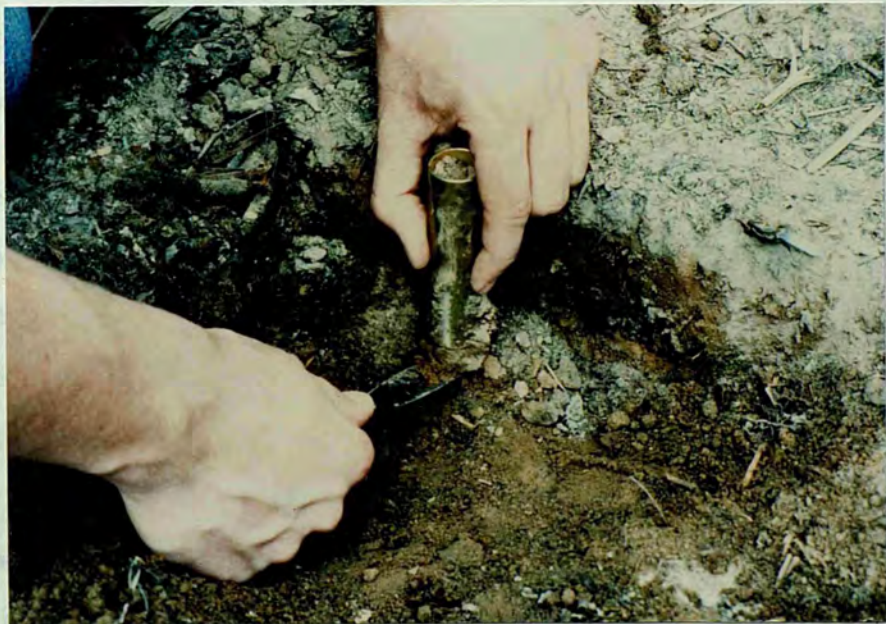
Collection of soil samples using tubes
