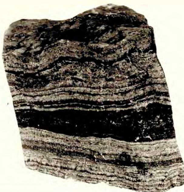
Plate 34. Hand specimen of laminated replacement-limestone, from the Soft Cap, Fossil Forest, Lulworth. X \frac{3}{4} . L. 101.
