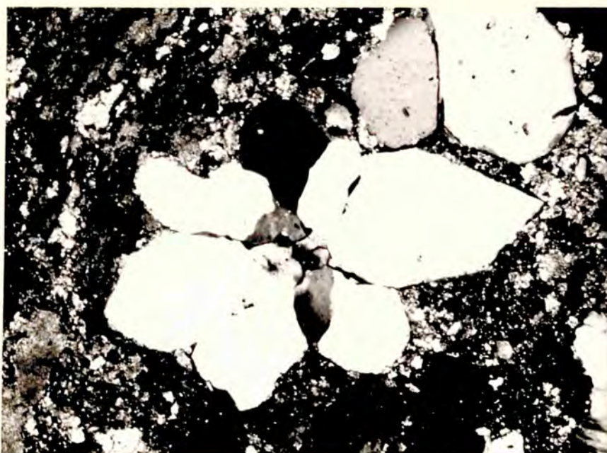
Plate 38. Rosettes of quartz crystals, Soft Cap, Worbarrow Bay. X. 460. M. 58.
