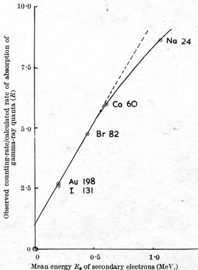
Fig. 2. Relationship between counting-rate and energy of secondary electrons in thallium-activated potassium iodide. Resolving time, 10  $\mu$ sec.; photo-multiplier voltage, 1,080; amplifier gain, 16,000; mass of crystal, 0.126 gm.
