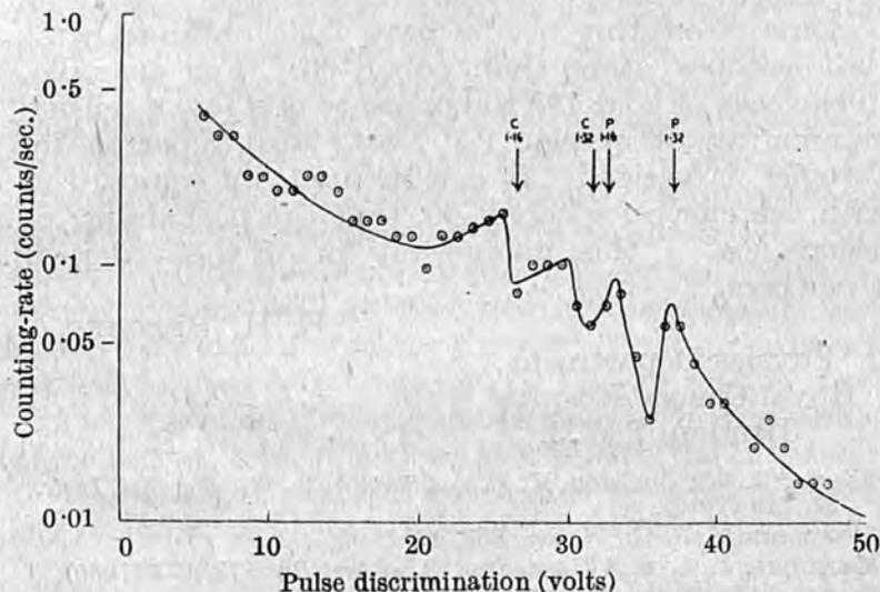
Differential counting-rates in calcium tungstate with 1 mC. of cobalt-60 at 1 m. Photomultiplier voltage 1,080; amplifier gain 1,600; mass of crystal 0.1244 gm.; resolving time 200  $\mu$ sec.
