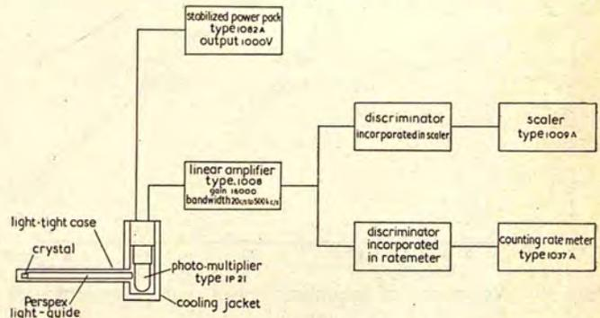
Fig. 4. Schematic diagram of scintillation counter
