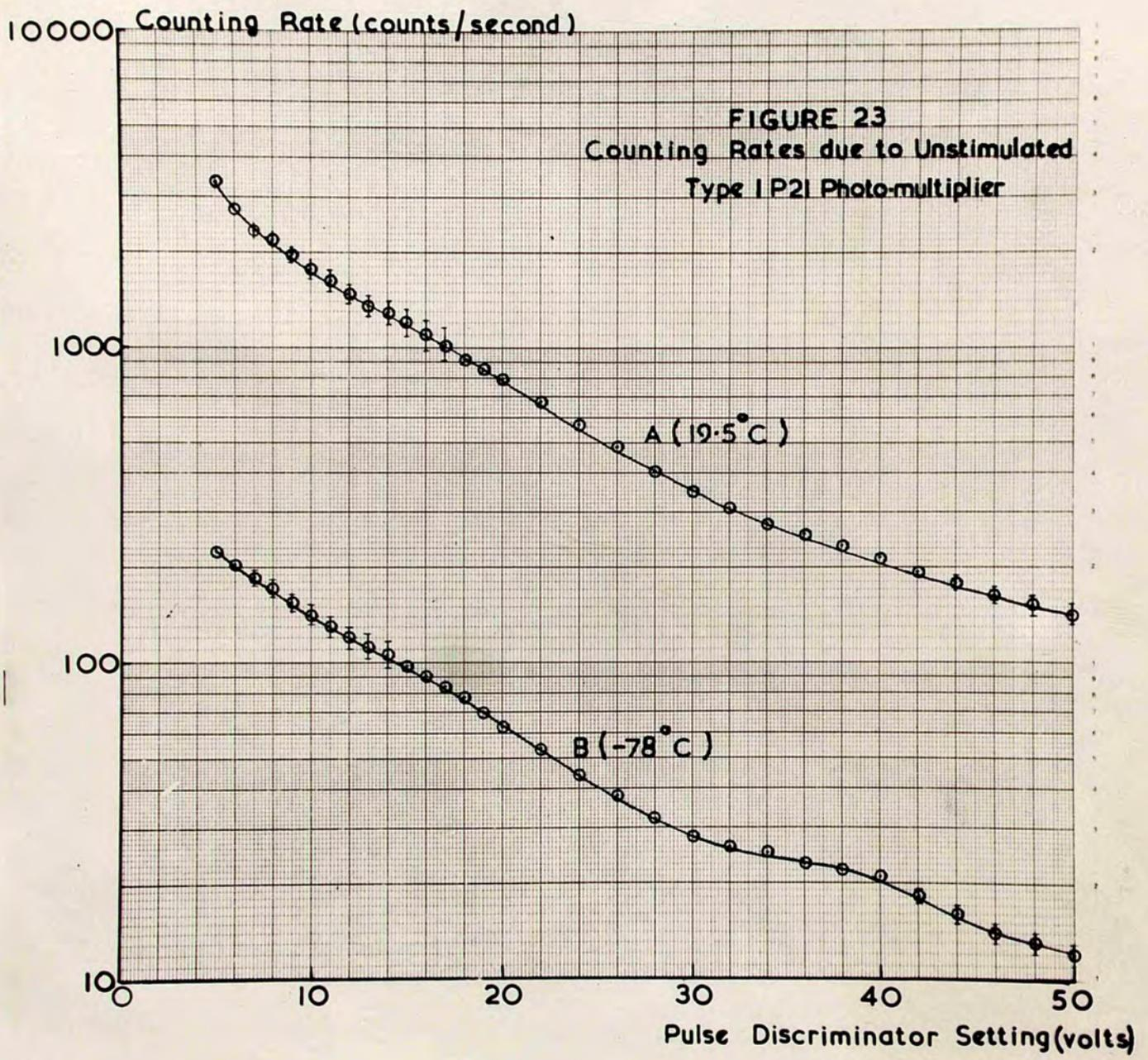
SECTION IV : EXPERIMENTAL RESULTS.1. STATISTICAL STUDIES ON THE TYPE I P 21 PHOTO-MULTIPLIER TUBE.(a) Photo-multiplier Dark Current Pulse Amplitude Distribution:
