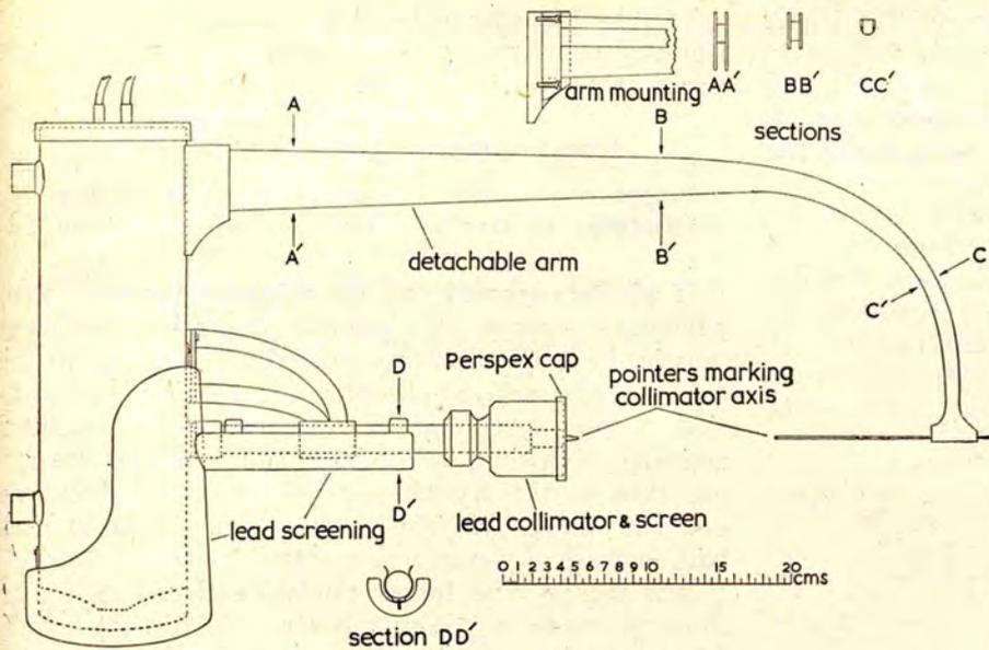
Fig. 2. Scintillation counter, external view
