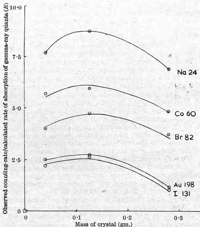
Fig. 1. Relationship between counting-rate and rate of absorption of gamma-ray quanta in thallium-activated potassium iodide. Resolving time, 10  $\mu$ sec.; photo-multiplier-voltage, 1,080; amplifier gain, 16,000
