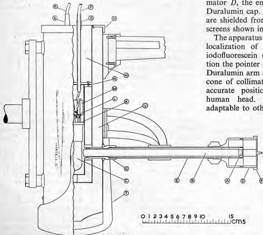
Fig. 1. Scintillation counter
