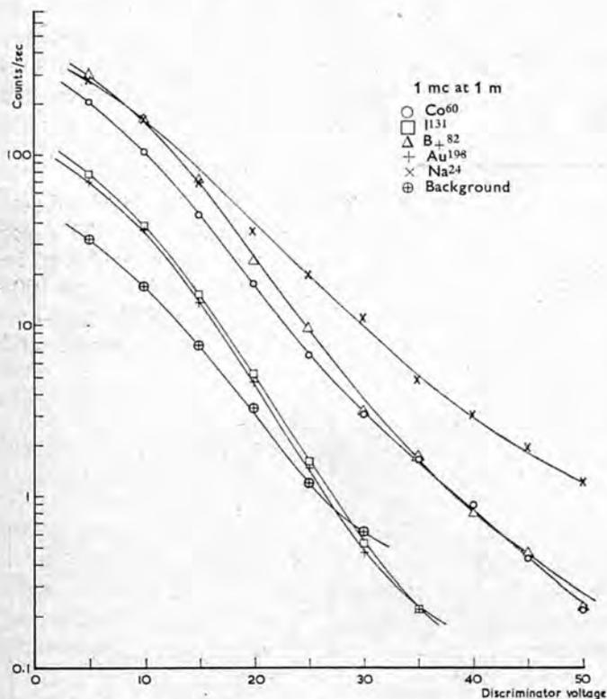
Fig. 6. Variation of counting rates with discriminator voltage
