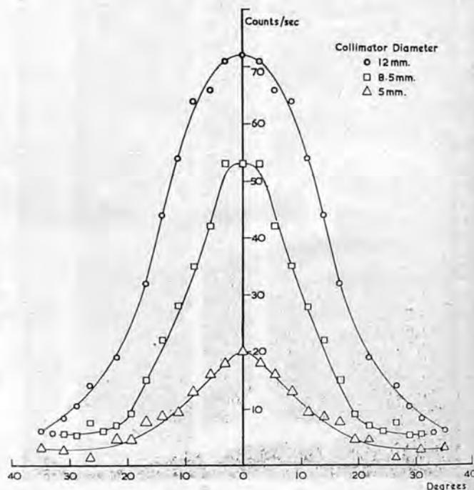
Fig. 7. Polar diagrams of counter for 1 mc of I<sup>131</sup> at 1 m
