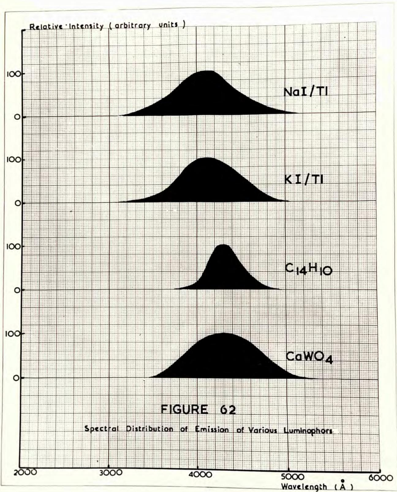
The spectra were examined with a micro-densitometer, and the blackening plotted as a function of wavelength. Because of the difficulty in estimating the radiation flux through the crystal, it was not possible to make absolute measurements of intensity of emission. The distributions were therefore plotted on an arbitrary scale, taking the peak intensity of emission as 100 in each case.
