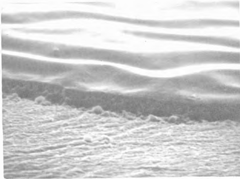
Figure 8.10. Electron micrograph of antenna metallisation. Magnification = 7500.
