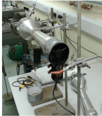
Fig. 2 The experimental set-up utilising the vane anemometer to measure the average velocity at the pre-mixer's outlet
