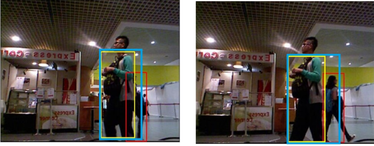
Figure 2: Occlusion search region: \Omega_{T_{search}}^i (blue line), \Omega_{T_{occ}}^i (yellow line), \Omega_{T_{obj}}^i (red line) .
