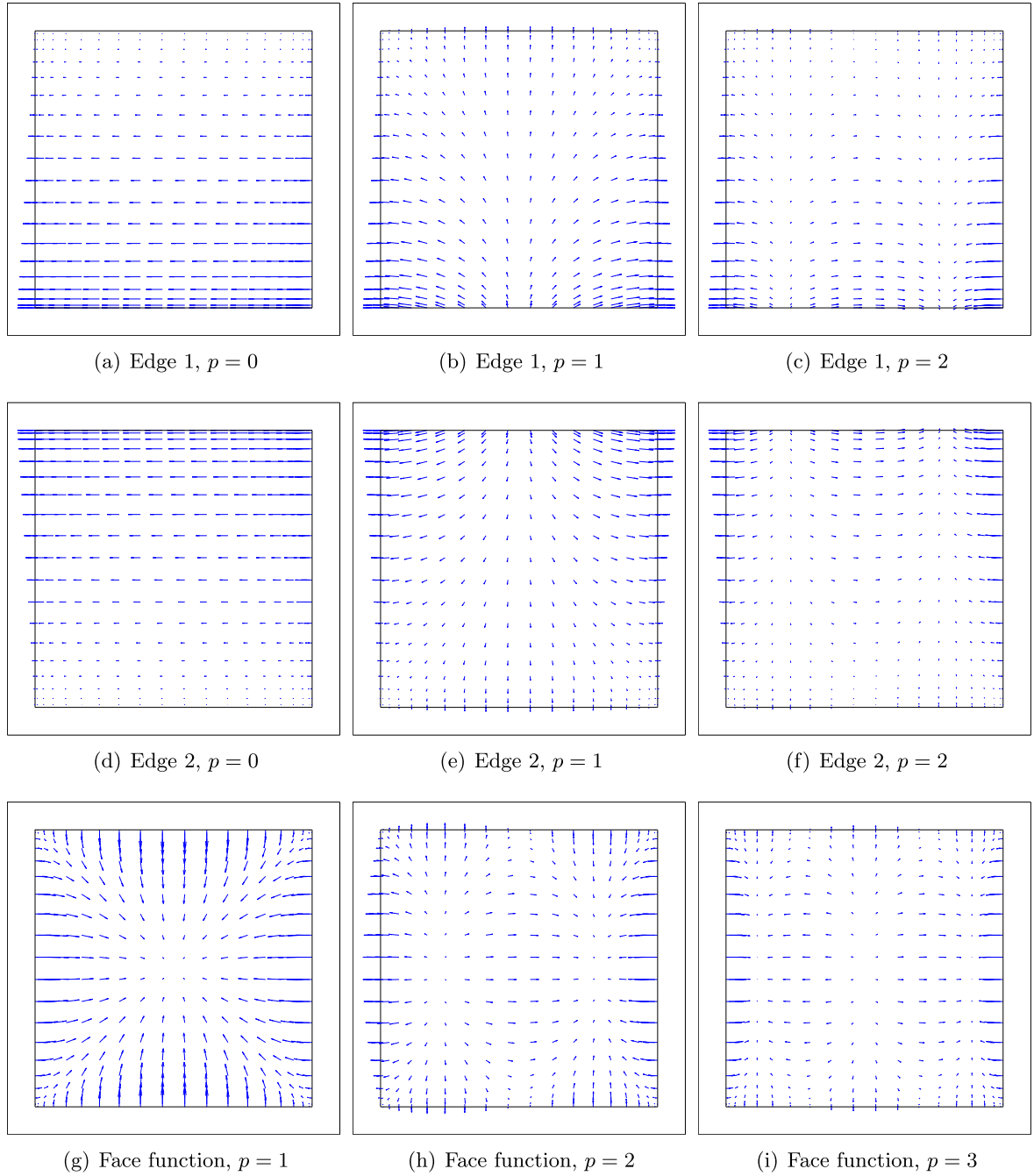
Fig. 2. An illustration of typical Nédélec edge- and face-based basis functions, restricted to a quadrilateral face. In (a)-(f) the edge-based functions are shown for two typical edges and polynomial degrees p = 0, 1, 2 . In (g)-(i) typical face-based gradient functions are shown for p = 1, 2, 3 .
