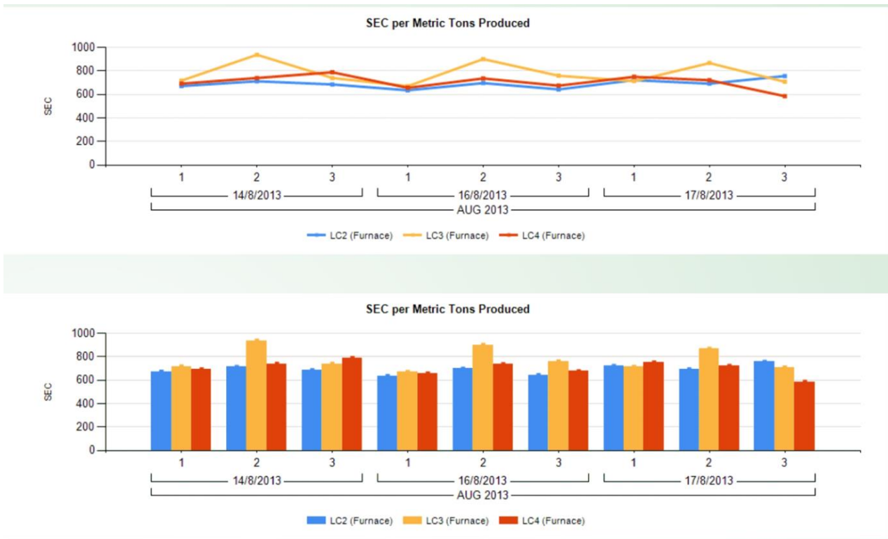
Fig.3. Specific energy consumption per tonne of melt produced is compared for three furnaces for a period of 3 days.
