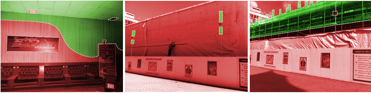
Fig. 1 Constraint maps of a sample snooker room wall (Left) and a construction scene (Center) with dynamic constraints (Right). The green region highlights valid camera mounting positions with invalid positions mapped to red. The construction scene images correspond to the right wall of the camera surveillance scene in Fig. 7. The focus region must be fully in view of the camera for a position to be considered as valid.
