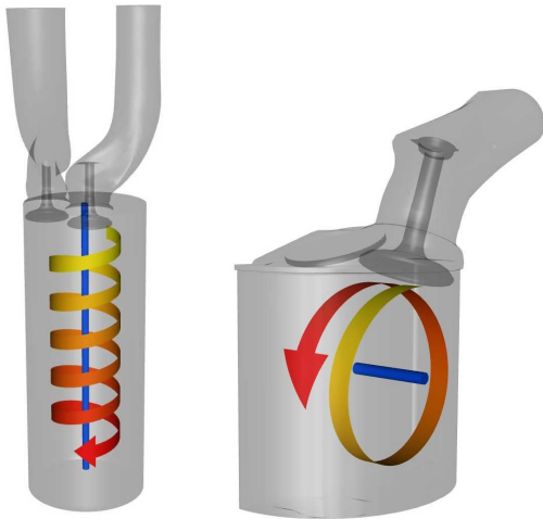
Fig. 1 (left) The swirling motion of flow in the combustion chamber of a diesel engine. Swirl is used to describe circulation about the axis aligned with the valve cylinder. The intake ports at the top provide the tangential component of the flow necessary for swirl. The data set consists of 776,000 unstructured, adaptive resolution grid cells. (right) Some in-cylinder flows require a tumble motion flow pattern in order to mix fluid with oxygen. Tumble flow circulates around an axis perpendicular to the cylinder axis, orthogonal to the case of swirl motion.
