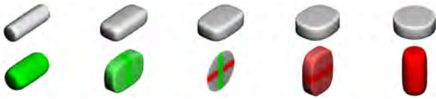
Fig. 5: A visual comparison of the superquadric glyphs (top) and our glyphs (bottom). From left to right, the tensor shown is linear degenerate, linear non-degenerate, neutral, planar non-degenerate, and planar degenerate, respectively. Our glyphs are based on the deviators, which highlight the difference and symmetry between linear, neutral, and planar tensors. Green and red represent linear and planar, respectively. The colored bands on the glyph's faces correspond to eigenvalues with the same sign (two negative, in the case of linear tensors, and two positive for planar tensors). The direction perpendicular to the bands are the non-degenerate eigenvectors, i.e., major eigenvectors for linear tensors (green) and minor eigenvectors for planar tensors (red).
