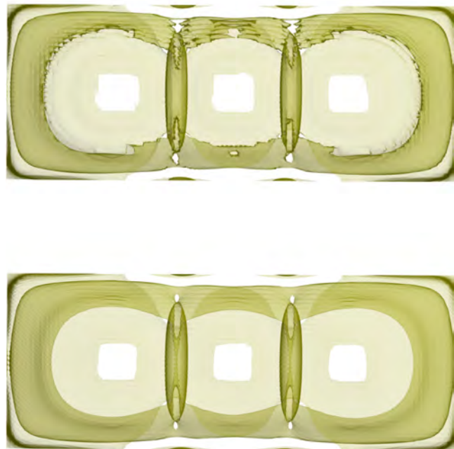
Fig. 3: This figure compares the neutral surface of the three ball simulation using the Marching Tetrahedra method (top) and the A-patches method (bottom). Notice that not only does the A-patches method better preserve geometry details such as the outline of the holes, it also reduces the topological errors caused by the Marching Tetrahedra method.
