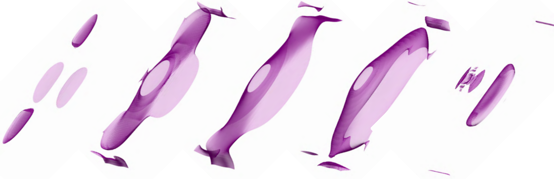
Fig. 11: The isosurfaces of the isotropy index with values at 0.70, 0.36, 0, -0.36, and -0.70 for the single sphere scenario in Figure 7.
