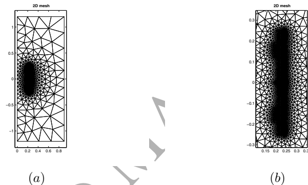
Figure 4: (a) Mesh of 6 820 unstructured triangular elements for \Omega^p for the eddy current problem and (b) A close-up showing the details of the coils, shields and OVC
