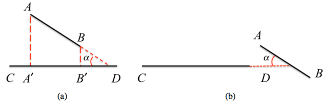
Fig. 4: The disadvantage of parallel measurement by angle: case (a) and case (b) cannot be distinguished.
