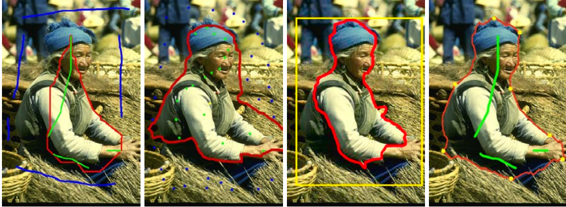
Figure 1. From left: Graph cut [1], Seeded Star Graph Cut [20], GrabCut [17], and proposed method. Red curve shows the segmentation result, blue for the background strokes, green for background strokes and yellow for the star point and the initial window of the Grabcut.
