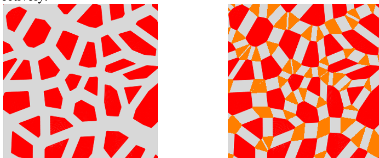
Fig. 2 (a), (b) and (c) are the 2D EBSD (Electron backscattered diffraction) experimental microstructural image of NPC Nickel with decrease in average grain sizes respectively. The decrease in average grain size shows the increase in number of triple junctions. Fig. 2 (d), (e) and (f) are the schematic views of two dimensional multiphase NPC model showing the increased number of triple junctions in NPC material as the grain sizes decreases. The blue circles, red lines and white polygons show the triple junction phases, grain boundary phases and grain phases respectively.
