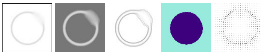
Figure 1.16: Diffused region force on weak edge - from left: the edge map, the stopping function g(\cdot) of edge map, the magnitude of its gradient \nabla g(\cdot) , the region segmentation map, and the vector map of the diffused region force \tilde{R} .
