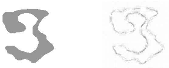
Figure 1.4: The doublet effect of the second term of equation (1.7)- The gradient vectors are all directed towards the middle of the boundary, which forces the snake into the valley of g(\cdot) .
