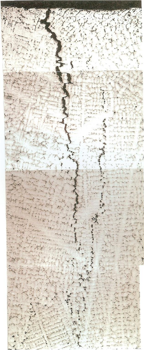
Figure 8: Cavity development along columnar grain boundaries during service of HK40 tube steel.
