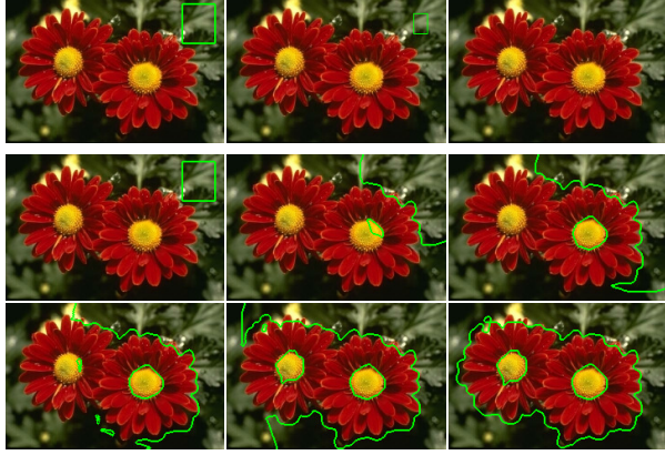
Figure 1. (1st row) Segmentation result using conventional level set; (2nd row and continuing on 3rd row) Results using proposed method.
