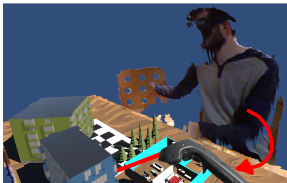
Figure 4: The user orbited left, so he can see a 3D reconstruction of himself and the chairs when looking to his right.
