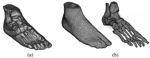
图1 (a)面模型,(b)软组织和骨骼的有限元网格模型 Fig. 1 (a) Surface model and (b) FE meshes of the encapsulated soft tissue and bony structures
