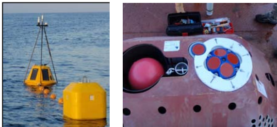
Figure 7. Wave buoy (left) and deep water ADCP (right) deployed at the Wave Hub site
