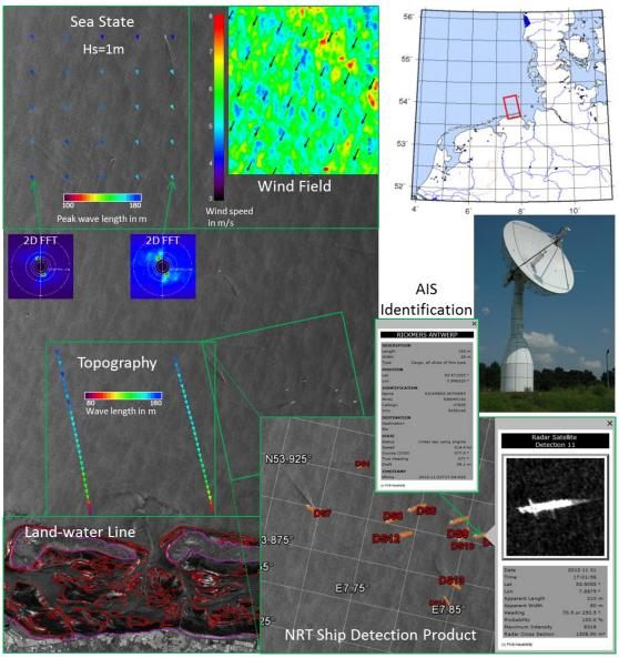
Fig 1: TerraSAR-X Stripmap scene with results provided by maritime NRT-value-adding-processors. Shown are wind field, sea state map (here swell from a different direction to wind), topography retrieval, ship detection results and land-waterlines (date: November 21, 2013) at the German North Sea Coast, © DLR 2013, Visualization of ship detection in Google Earth.
