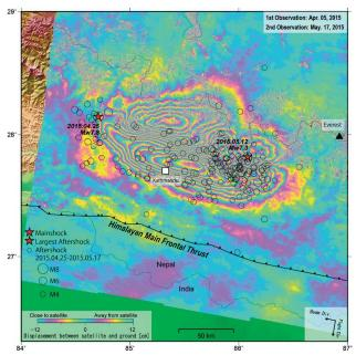
The 2015 Nepal(Gorkha) Earthquake: Crustal deformation detected by ALOS-2 data Analysis by GSI from ALOS-2 raw data of JAXA
