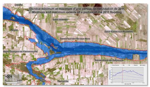
Fig 2: Exemple of the animation made with the EO-1 & 16 RADARSAT-2 images. The maximum flood extent is shown in red. Credits: CSA, MDA, NASA, USGS, Effigis.
