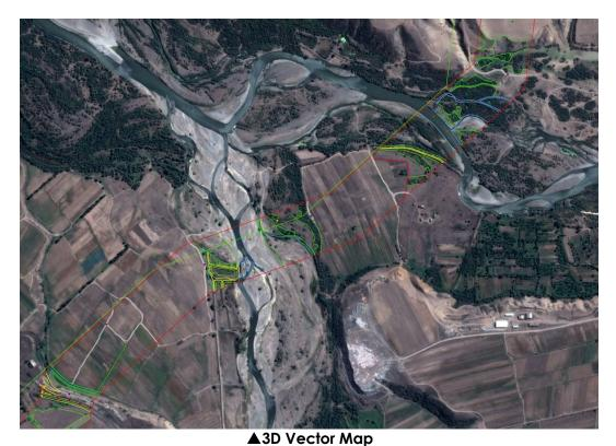
Topographic feature extraction at 1/5,000 scale
