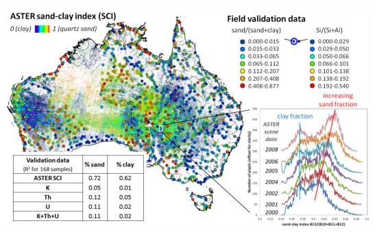
Fig 3: ASTER map of the proportion of sand to clay size material (SCI) validated using field sample analyses of particle size and Si and Al geochemistry. Table (bottom left) provides regression statistics for field sample data. Yearly (2000-2008) histograms (bottom right) of the ASTER SCI for an area near Lake Eyre.
