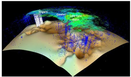
Fig 2: 3D oblique view of the Australian crust that combines the surface clay mineral composition from ASTER (warmer colours are illite-montmorillonite and cooler colours are kaolinite) with the base of crust (MOHO) and seismic activity (blue dots).
