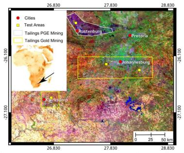
Fig 1: Landsat 8 composite (R: 2200 nm, G: 860 nm, B: 550 nm) of areas affected by gold and platinum mining and associated tailings sites around the greater Johannesburg and Gauteng area, after Mielke et al., 2014. ETOPO-1 inset map (data courtesy NOAA) for reference. Please note that only the future Sentinel-2 will have a swath large enough to cover the whole area in one data acquisition. Whilst the here presented composite is a mosaic of four Landsat-8 scenes.
