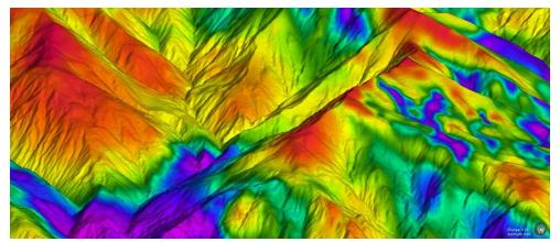
Fig 2: Analytic Signal Vertical Integral (ASVI) Airborne Magnetics draped over AW3D- Shaded Relief (©NTT Data, RESTEC/Included©JAXA)
