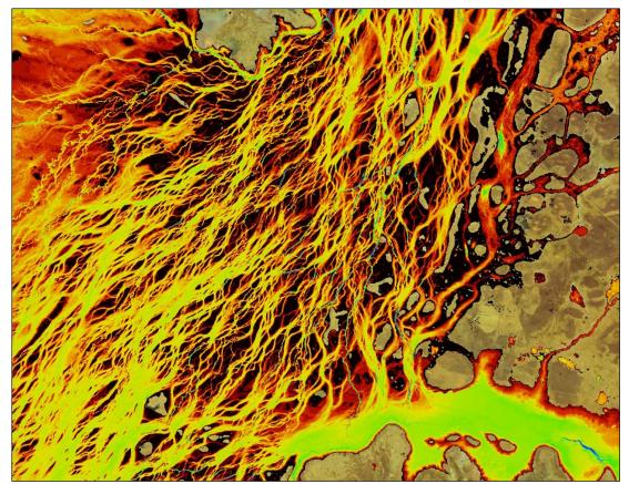
Fig 2: The braided river network of Coopers Creek in south-western Queensland as depicted by WOfS. The colouring indicates the frequency of inundation (see Figure 1 for legend), with blue areas showing permanent water holes in an extremely hot and arid region. These braided river networks are difficult to map by topographic methods.
