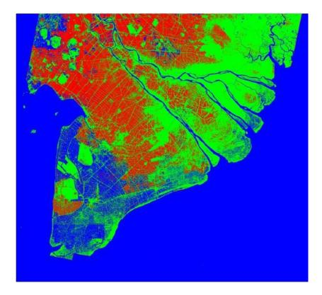
Figure 2: Rice grown area (in Red) for the Winter Spring Rice season (December 2014-March 2015). This is an unprecedented mapping results of a large area ( $300 \times 300 \text{ km}$ ), at a resolution of 40 m (it is possible to have results at 10 m), and near real time acquisition. The data are available the day after acquisition and processing can be done during the day. A map can be provided every 12 days to show the rice crop growth in the region.
