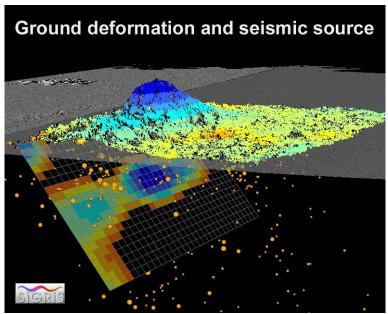
Fig 1: Ground deformation map and earthquake source model generated for a magnitude 5.8 earthquake on May 29th, 2012 in the Emilia region in Northern Italy. The post-event image was acquired 5 days after the earthquake, and the source model was generated in 2 hours and validated using seismological and GPS data. These products can be used to define the event scenario.
