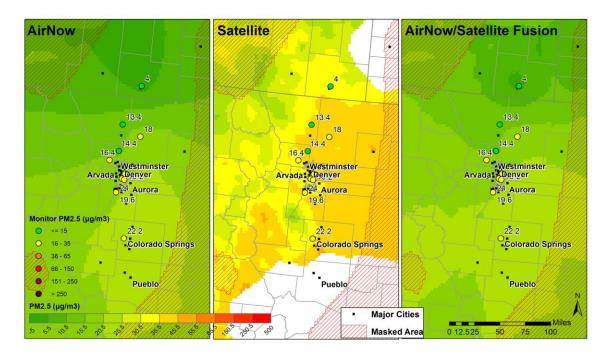
Fig 1: Example of ASDP data fusion product. The image shows 24-hour average PM2.5 ground concentrations from AirNow (left panel), satellite-estimated PM2.5 levels (middle panel), and the fusion of satellite and ground monitor data (right panel). The dots show monitor locations and concentrations. Colors reflect the AQI, and white areas in middle panel indicate areas obscured by clouds. Image credit: ASDP.
