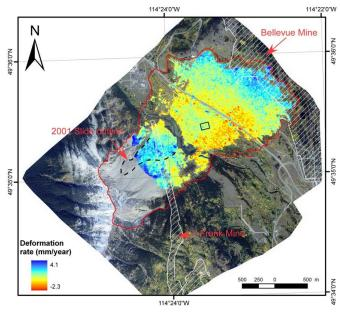
Fig 2: Crowsnest Pass. In conjunction with studies being undertaken by the Alberta Geological Survey (AGS) on unstable slopes on Turtle Mountain, site of the Frank Slide, InSAR technology was utilized to map subsidence of the ground overlying the abandoned coal mine workings. By utilizing Radarsat-1 Fine beam data from fall 2004 to summer 2006, many thousands of coherent targets were identified above the mines and a map was produced showing the rates and patterns of deformations.
