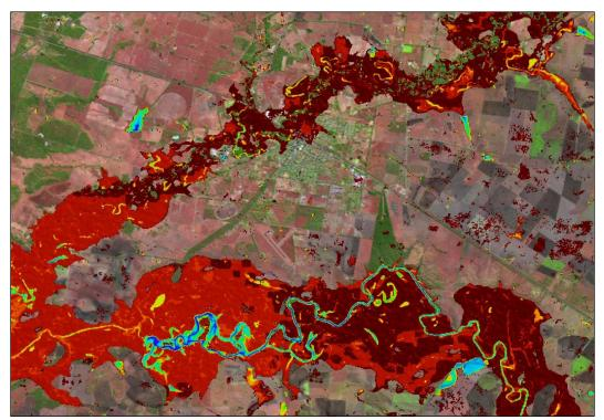
Fig 4: The WOfS product in the area of Chinchilla in southern Queensland. The blue areas indicate where water is a usual occurrence, while the red areas indicate unusual water observations such as caused by flooding. Here the red area spills into the Chinchilla township due to the extreme flood conditions from December 2010 (see Figure 1 for legend).
