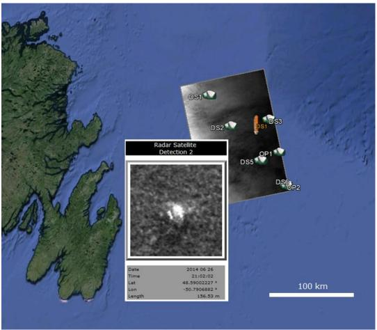
Fig 2: Semi-automatic iceberg/vessel detection report (near Neufoundland, Canada), based on TerraSAR-X (date June 26, 2015), © DLR e.V. 2014, Distribution Airbus DS. Visualization in Google Earth.
