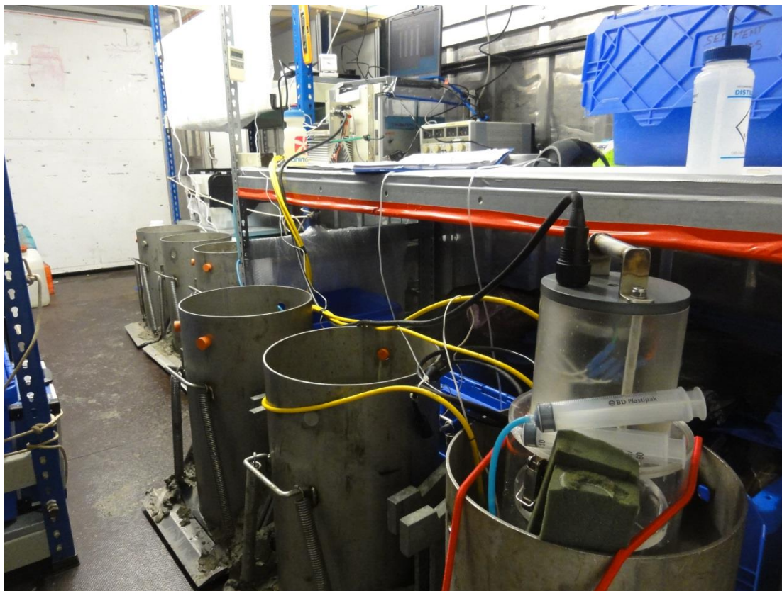
Figure 1: Core Mini Flume in place during the resuspension experiments from Benthic A.
