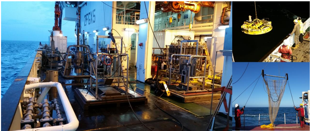
Figure 1: A variety of benthic sampling equipment was deployed on DY021: (main picture from left to right) SMBA 0.5m 2 box-corer, NIOZ 0.1m 2 corer, Sediment Profile Image (SPI) camera, ChemSPI; (top right) Voyager II benthic in situ flume; (bottom right) 2m Jennings Beam trawl.
