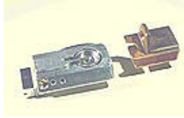
Fig. 16. SEM cryo-stage specimen carrier for frozen sections. The original specimen sledge for bulk samples was milled-out and a block inserted to hold a tip from a Philips TEM specimen rod. This held the grid carrying the frozen sections. A copper ring under the tip acted as a cold support for the specimen. The object at the right is a copper cover that was put in place when the sections were loaded into the holder to protect them as they were put into the SEM. This was removed in the cryo-stage airlock by means of a "sky-hook" before the specimen was inserted into the main stage of the microscope.
