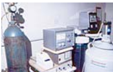
Fig. 22. Freeze-drying set-up in Room 61. Nitrogen bottle at left for purging and venting the system, electronic control system in the centre with the white switch box for the liquid nitrogen pump, Anavac mass spectrometer below, analogue thermometer at top above the feed-back power control box for the heater in the specimen stage. The coating unit/freeze-drier is seen behind and the liquid nitrogen dewar for the freeze-drier is at the right. The liquid nitrogen pump is inserted into the top of the dewar. Photo taken in 1989.
