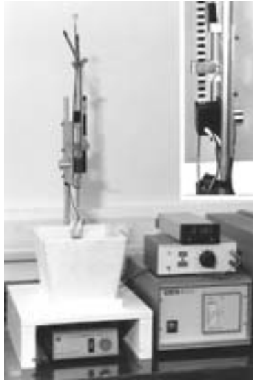
Fig. 13. The original bench-top plunge freezer with magnetic stirrer below, coolant temperature feedback control (at right, below), coolant power supply and digital thermometer above. The inset shows the plunge scale and the infra-red sensor that recorded plunge velocity. Photos taken 1985.
