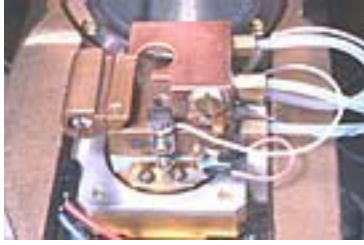
Fig. 15. Cryo-stage for the 35C SEM. The anti-contaminator is uppermost, cooled by liquid nitrogen passing through the plastic tubing, with a cut-out (near left) for line-of-sight access by the x-ray detector. The hole through the stage can be seen, for transmitted electron imaging of frozen sections. The cartridge heater is seen at left, with red and blue power leads. The clear Perspex Faraday cup (nearest camera) with a white-coated lead is for electron beam measurement during quantitative x-ray microanalysis. This stage was made by David Purse in the MBA Engineering Workshop.
