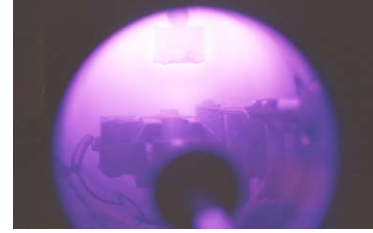
Fig. 17. View of a frozen specimen being sputter-coated with gold in the SEM cryo-stage airlock. The cold pre-stage is seen in the centre of the photo, with copper braid attached at left for conduction-cooling by liquid nitrogen. The sputter head is at the top. This was made in the MBA Engineering Workshop. The blue colour is due to the ionised argon plasma that is integral to this process. Cryo-fracture could be done with a scalpel blade that was pre-cooled in a slot in the cryo-stage. Specimens could also be coated using a carbon arc or carbon fibre and also by other metals using a tungsten filament for evaporative coating. Photos taken 1985.
