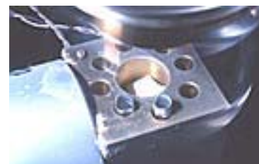
Fig. 24. Close-up view of the freeze-drier specimen stage. Two specimen tubes are seen, full of liquid nitrogen at this early stage. These were simply aluminium foil tubes formed around a drill bit. There are eight specimen stations plus a central station where specimens were parked while the tubes were loaded. A thermocouple is clamped at top left to control the power supply to the liquid nitrogen pump. A free thermocouple is inserted into an empty specimen station to monitor its temperature and this feedback controlled the cooling. Photo taken in 1989.
