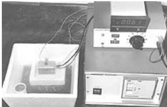
Fig. 26. Cryo-mounting set-up for attaching frozen specimens into SEM cryostage supports prior to quantitative x-ray microanalysis. The digital thermometer is showing -61\text{ }^{\circ}\text{C} which is the operating temperature for the cryo-glue. Photo taken 1986.
