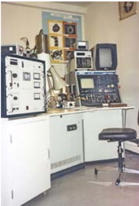
Above: Fig. 12. JEOL 35C SEM in its original location in the basement, with the cryo-stage attached to the airlock and the brown dewar of the x-ray detector at the rear of the column. The x-ray system was controlled very easily by the small keypad at the right side of the microscope console. The microscope was moved upstairs to Room 57 in 1988.
