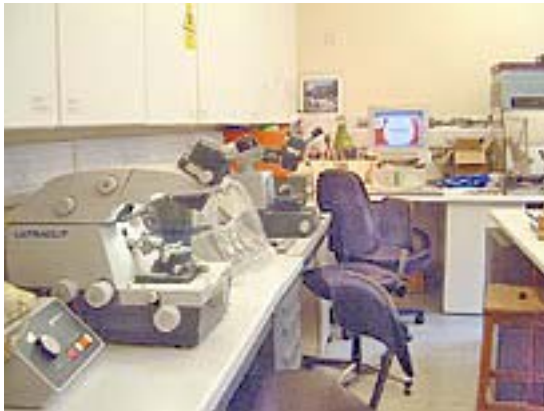
Fig. 28. EM Prep Room (Room 55) after relocation in 1988, showing the two ultramicrotomes, the Reichert Ultracut (nearest) and the OmU3.
