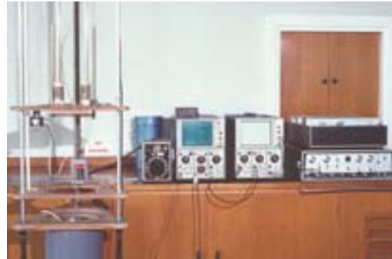
Fig. 14. Experimental setup with the deep plunger, coolant heater supply (Variac), thermocouple signal display oscilloscope with digital thermometer above, amplifying oscilloscope for xy signal plotting (plotter at top right), and transient recorder (at bottom right) in the old Lecture Hall. This setup was also used originally with the bench-top plunger (left). Photo taken 1990.
