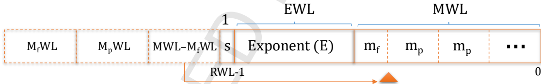
Fig. 3. General scheme of the double mantissa representation in fixed register of RWL length.
