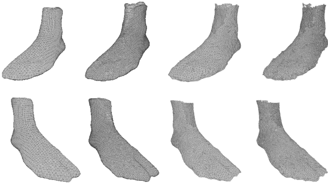
Fig. 13. Reconstructed models of a real human foot (left) acquired using a 3D scanner. From left to right: reconstructed model using Poisson (around 10,000 faces), using Poisson (around 30,000 faces), using GNG (5,000 neurons and around 10,000 faces) and using GNG (14,000 neurons and 30,000 faces).
