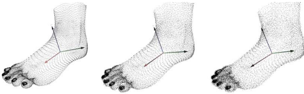
Fig. 6. Synthetic foot with different levels of Gaussian noise. From left to right: \sigma = 0 ; \sigma = 1 ; \sigma = 1.5 ; (millimetres)
