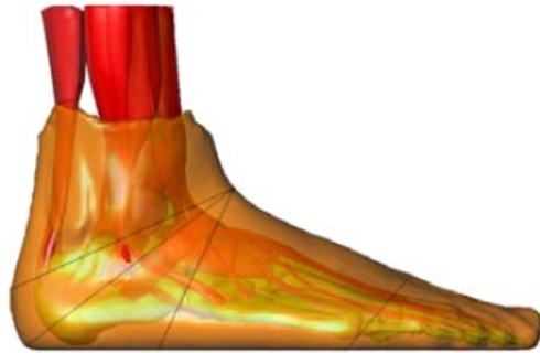
1 2 Fig. 15. Different curves whose perimeter measurement are used to manufacture custom footwear.
