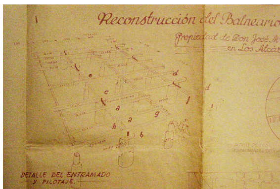
Figure 3: Layout of the cleats or marranos and the bolsters. Costas Murcia Archives. File C 302 MY San Antonio, Los Alcazares sea bathing resort.
