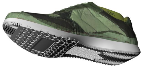
Fig. 59 - Sole prototype and last
