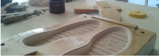
Fig. 48 - Prototype and plaster mould (lower cover)
