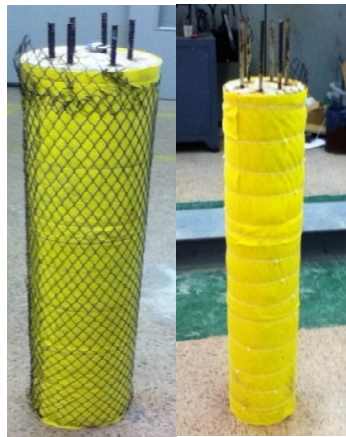
Figure 1. Anodic system composed by a Ti-RuO 2 mesh embedded between two absorbent polymeric layers, wrapping a reinforced concrete specimen. Adapted from [24].
