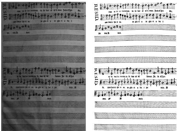
(a) Perspective-corrected image (b) Perspective-corrected image binarized by using Otsu's method
