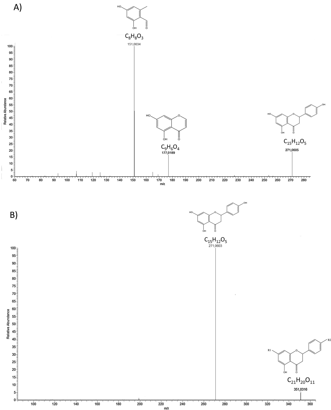
Fig. 2. MS 2 spectra of naringenin (A) and naringenin-sulfate (B). Naringenin-7- O -sulfate would correspond to R1 = OH and R2 = SO 3 H and naringenin-4- O -sulfate to R1 = SO 3 H and R2 = OH.
