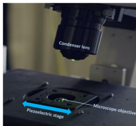
Figure 3: Central part of the microscope used in the Optical Trapping Lab, evidencing the movement of the piezoelectric stage, and the location of the microscope objective lens and the condenser lens of the force measurement device.
